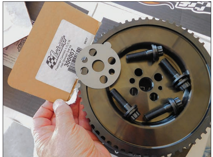
The Fluidampr 300007 High Strength Bolt Kit was my choice for fasteners. The kit consists of high performance ARP bolts and chamfered washers. Fluidampr adds the diamond impregnated friction washer for superior clamping. This kit will handle up to 700 horsepower and 1250 foot-pounds torque. My engine puts out half that power. The Fluidampr will stay in place!
