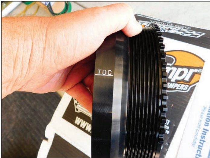
This is the new design damper for 2003-2007 Cummins engines. The chamfer seen at the inside edge is the clearance necessary to easily remove and install the drive belt. The change makes belt service in the field quick and eliminates the need to remove the damper.
