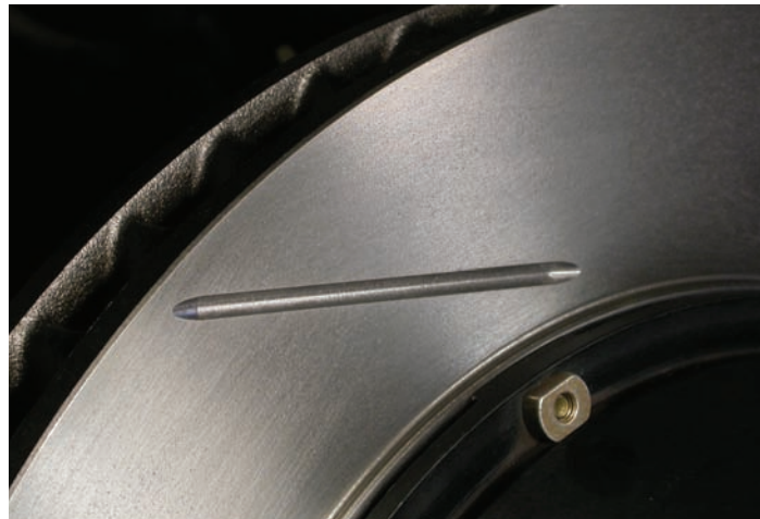
A typical rotor before bed-in. Note the clearly defined machining marks on the rotor face.
