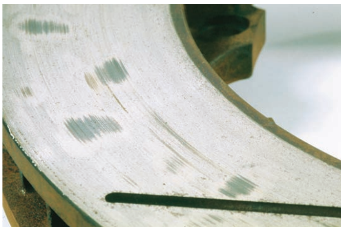
A rotor which has been exposed to an overheated brake pad. Note the friction material deposits on the face.
