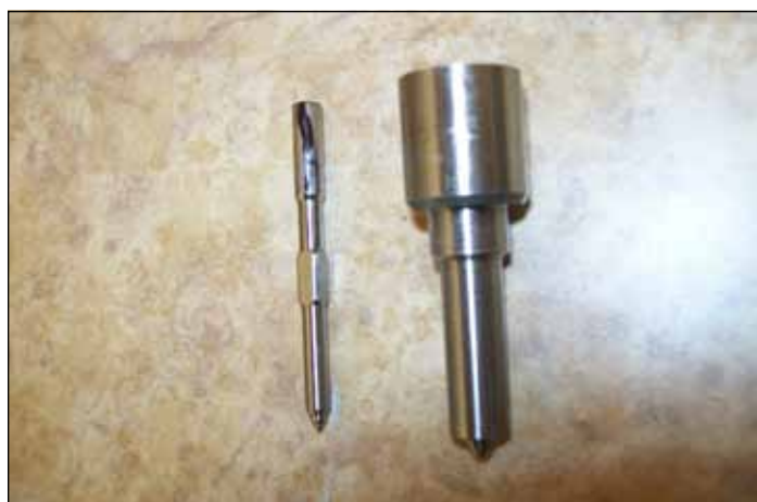
72i12. Pintle with Magic Marker stripe, showing inadequate clearance for the nozzle.
