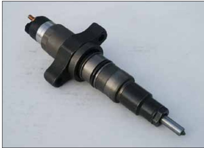
72i3. Bosch injector for the HPCR system. The extra height of the injector for the new common rail system, compared to older style mechanical injectors, accommodates the electrical control mechanism to open and close the injector. Prior designs on our Turbo Diesels used fuel pressure to open and close the injector.
