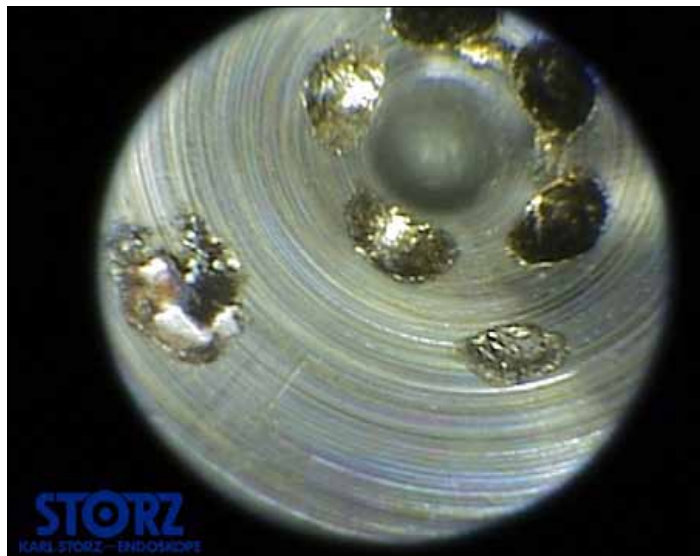
72i10. Borescope view of a poorly manufactured nozzle by an EDM process
