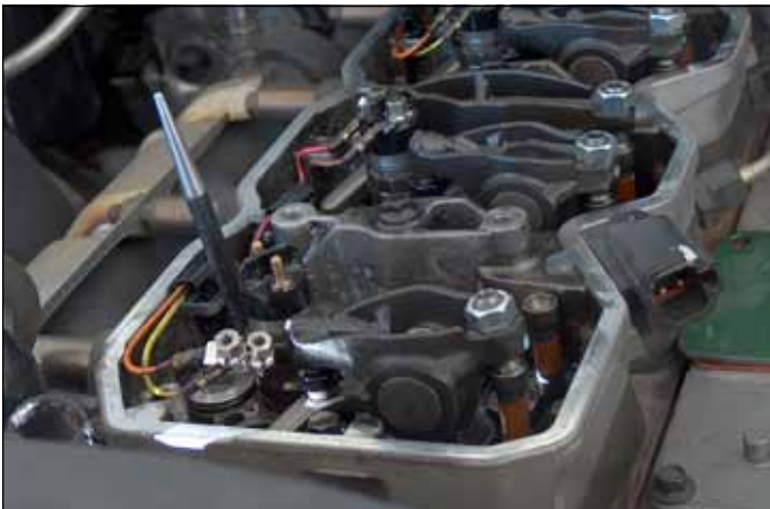
72i22. Common-rail engine with the "lady foot" injector puller positioned to lift #1 injector. (The exhaust rocker, injection line and connecting tube were removed first.)
