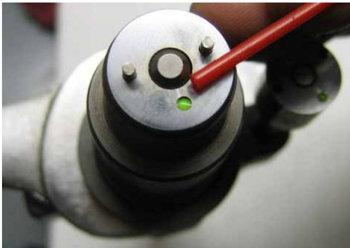
72i15. Cracked injector body
