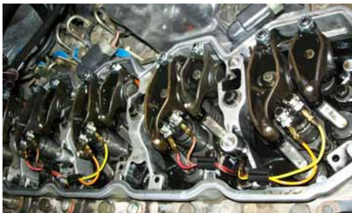
72i6. The rocker lever housing installed on an engine, with injector wiring shown for cylinders 1-3.
