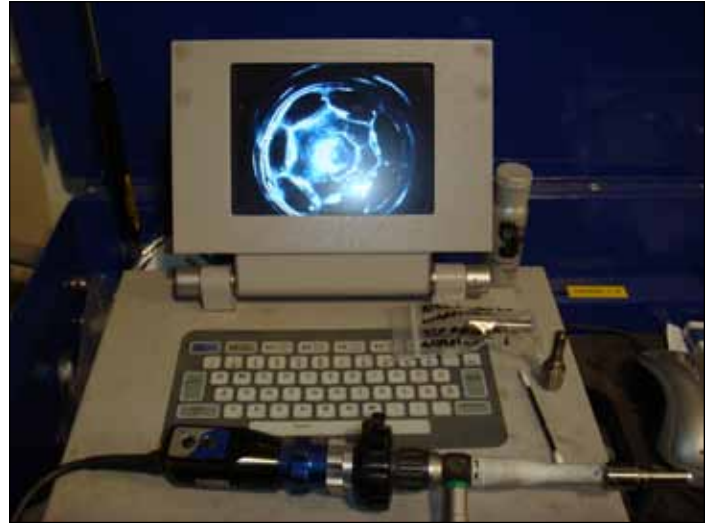
7218. Borescope on-screen view of the inside of an extrude honed 12-valve injector nozzle
