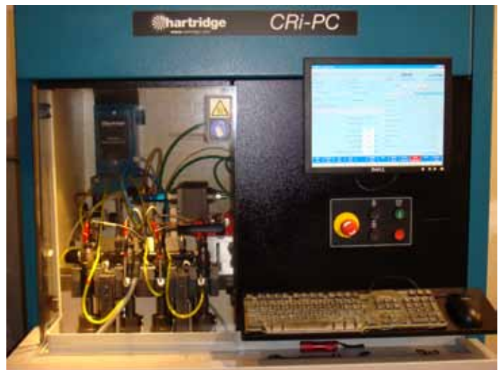
7219. Hartridge injector tester to determine leakage, flow rate, and response time
