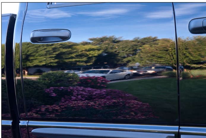
Figure 8: Paint perfection achieved with 4-step machine polish followed by "Best of Show" wax.
