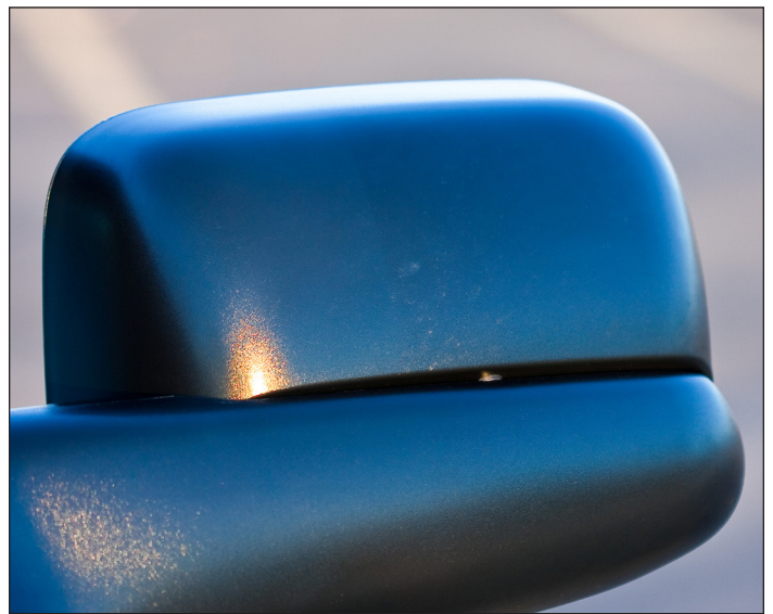
Figure 12: Rearview mirror after using Griot's 3" random orbital fitted with the yellow scrubbing pad (left side). The right side was cleaned with the same pad, only by hand.
