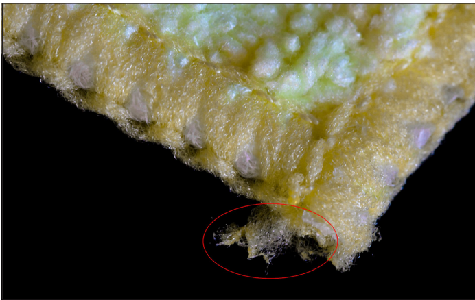
Figure 3: Costco cloth edge weave. A hard, melted portion on the corner (circled) has separated from the cloth, introducing some risk of scratching the paint. This cloth also shed some fibers when I shook it, unlike the Griot's cloth.
