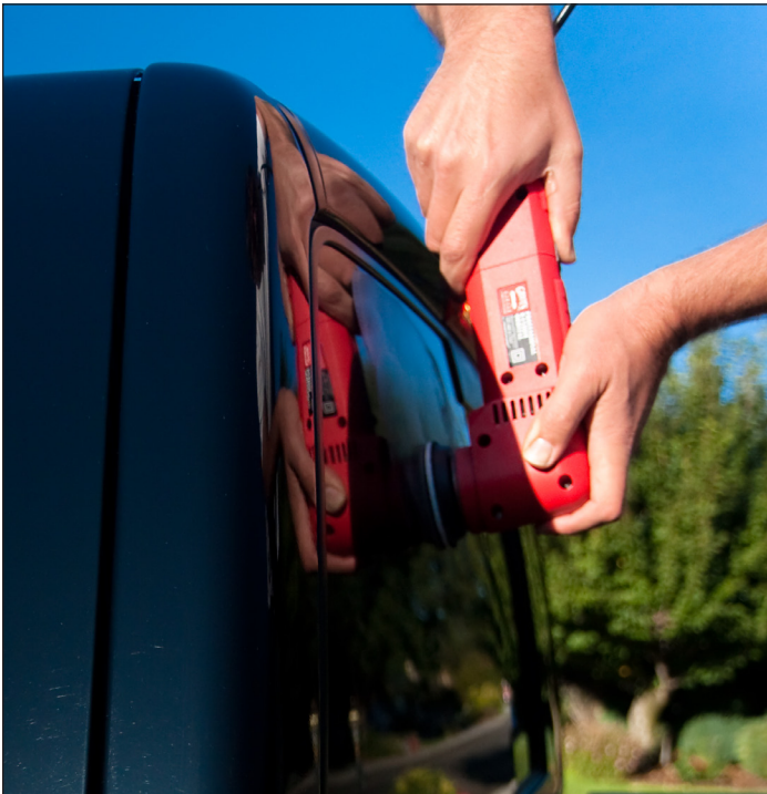
Figure 10: Polishing glass using the 3" random orbital, the white glass polishing pad, and Griot's glass polish.
