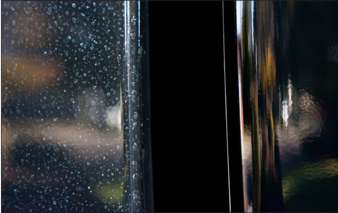
Figure 16: Machine Polish 4 (right side) takes care of new water spots that washing and Speed Shine could not.
