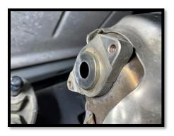
Before installing the new injector, you will want to make sure that the mating surface of the opening is clean. I ended up using a razor blade, scraped away the remaining fiber gasket material and finished it with a small sanding pad.
