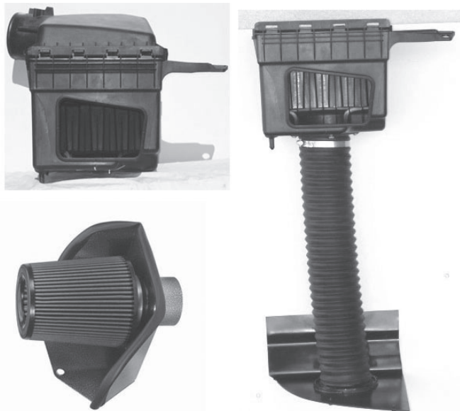
Stock Sealed Air Box (Upper Left), aFe Semi-Heat Shield Air Box (Lower Left), PSM Modified Sealed Stock Air Box (Right)
