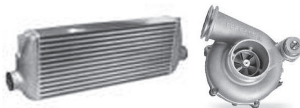
The best mass airflow enhancers: Intercooler (for increased air density) and turbocharger (for increased airflow)
