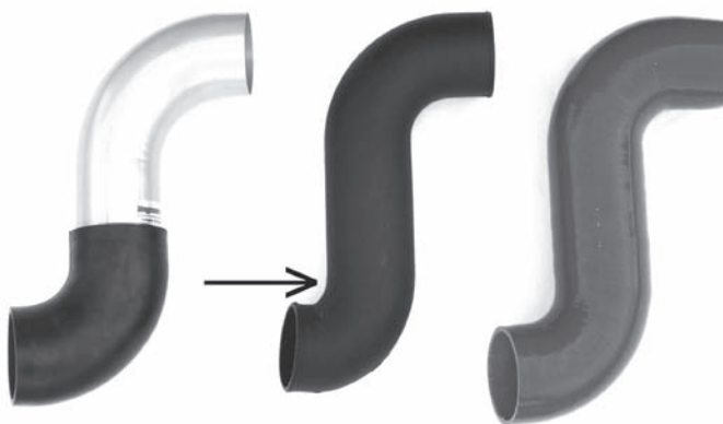
aFe steel/rubber Torque Tube (Left), aFe plastic Torque Booster tube (Middle), DPP silicone rubber Cool Tube (Right). Note tight bend in plastic tube (arrow) which increases air flow restriction
