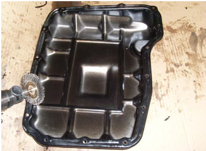
Cleaning the RTV from the 68RFE transmission pan.
