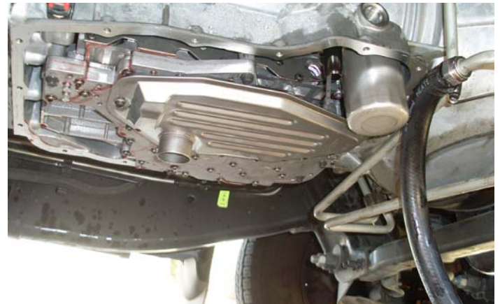
The bottom cooler line is the return-to-transmission line. Remove it with a 1" open end wrench. Clamp a 3/4" ID hose over the threaded barb and direct the fluid into a 5-gallon bucket.
