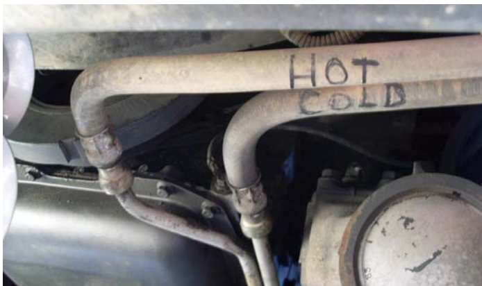
A view of the transmission lines from the front of a Second Generation truck. Follow the "cold" line back to the transmission cooler and disconnect the line at the junction point. Attach your purge hose to the metal flare at the transmission cooler.
