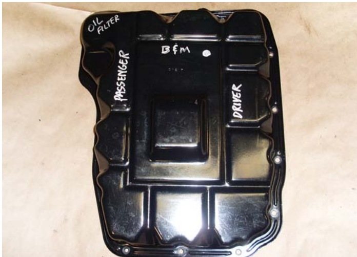
From my study of the internal parts of the 68RFE, I determined that the best place for the drain plug was the location that I marked "B&M."
