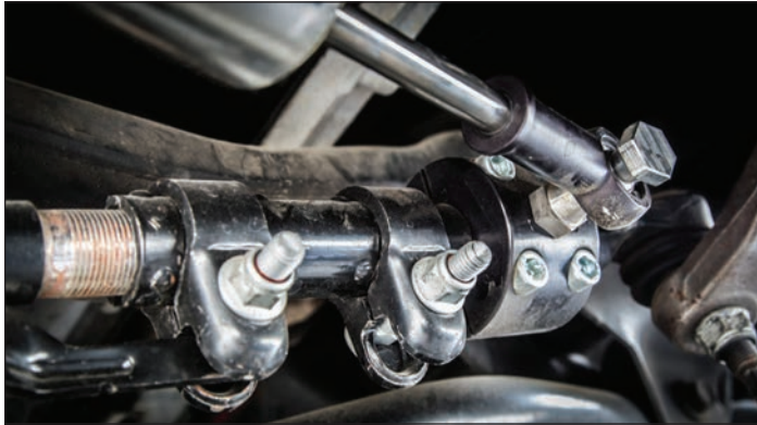
Figure 12: Installation of the Carli Suspension "High mount stabilizer" required a new clamp to accommodate the new tube diameter.
