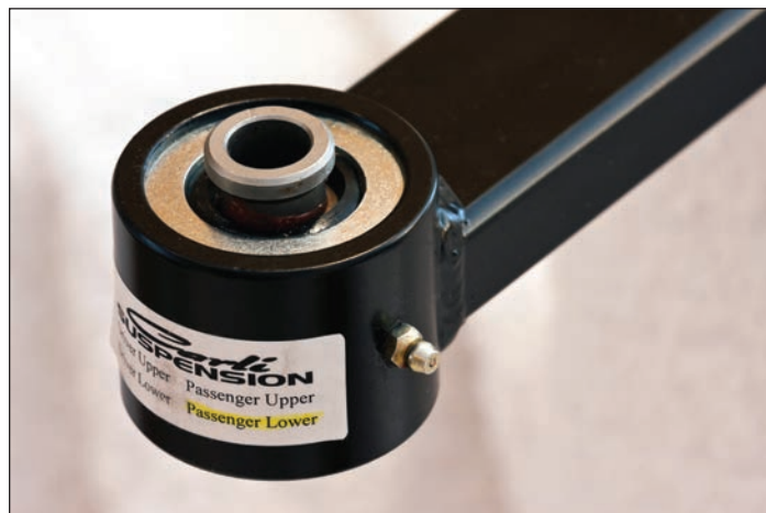
Figure 2: Carli suspension lower control arm, installed in 2012. The serviceable bearing eliminated the friction caused by the rubber bushings in the factory control arm.
