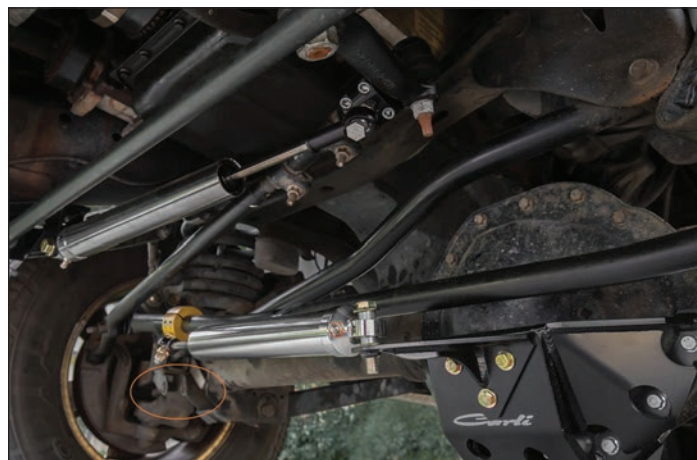
Figure 3: My (Issue 87) Installation of the Carli Suspension "Dual opposing steering stabilizers." Without using the factory mount point, the lower stabilizer is located above the bottom of the axle tube, reducing the risk of damage in off-road situations.
