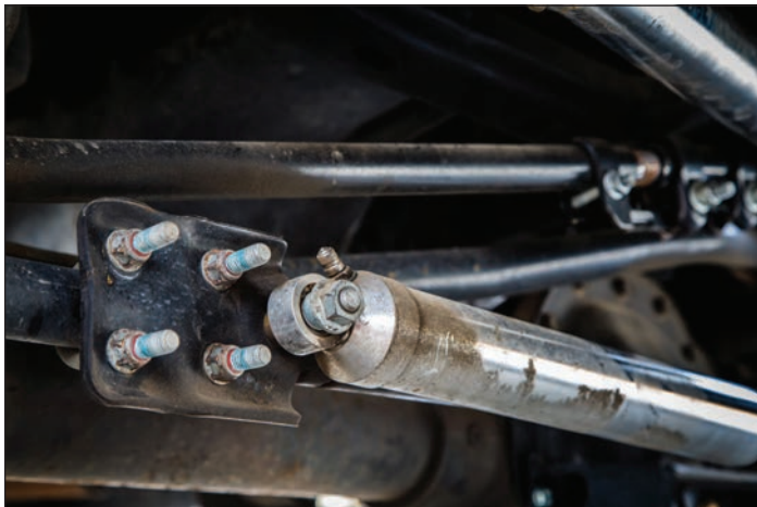
Figure 13: The Carli Suspension Low-mount stabilizer utilizes the factory supplied clamp, repositioned to the correct location per instructions from Carli Suspension.
