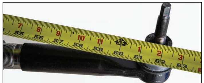
Figure 9: pre-adjusting the length of the new tie rod before installation.
