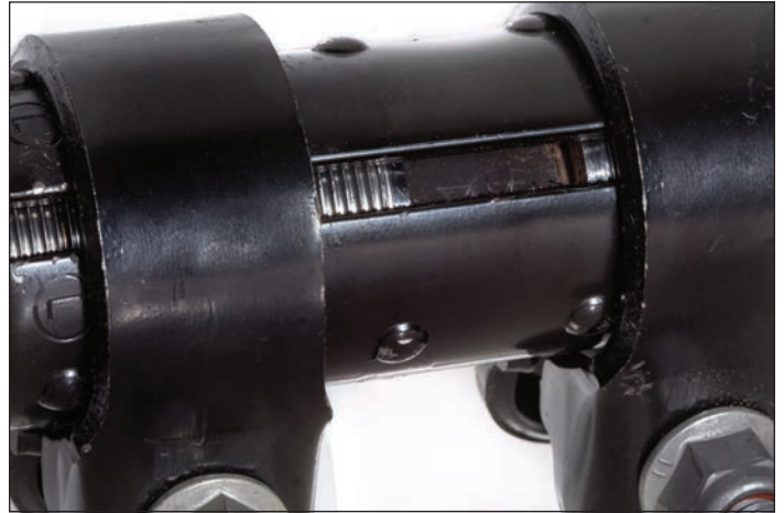
Figure 11: The adjustment collar on the newest T-style steering system. Note the inner mechanism in between the two threaded halves. This prevents the right hand tube from rotating along with the adjustment collar.
