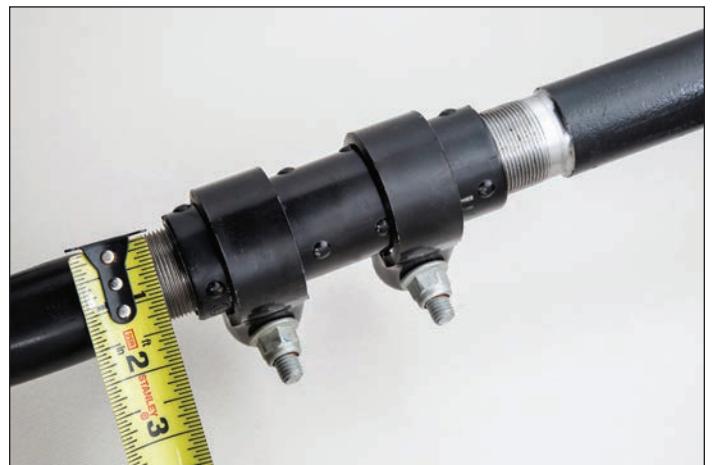
Figure 7: T-type steering system is made with 1.5" diameter tubing, and is considerably more robust than the older, Y-type steering system. The new system is over five pounds heavier.
