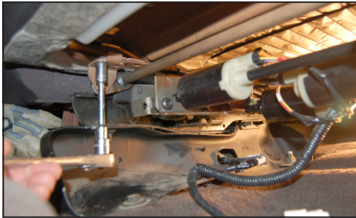
'94-'02 Truck: Removing the seat bottom frame.
