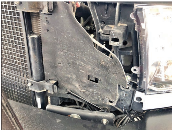
Combined with the grille, removing this wind flap made it much easier to fit a tube on the radiator drain.
