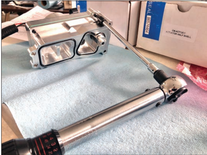
Assembling the new actuator upgrade kit from City Diesel.
