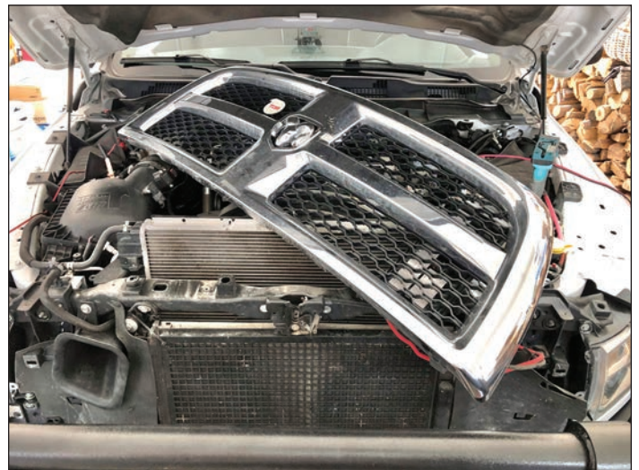
Pulling the grille was optional, but I prefer fewer knuckle scrapes, hassles, and better access.
