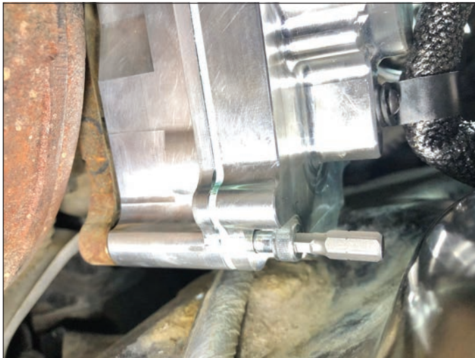
Miniature 5mm hex bit, turned by a 1/4" box-end, was a much better solution, as suggested by City Diesel.
