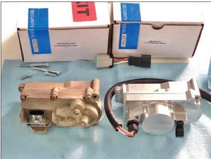
Factory Holset 6.7L VGT actuator left, and new City Diesel replacement on the right.
