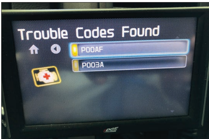
Telltale codes for a failed turbo actuator.
