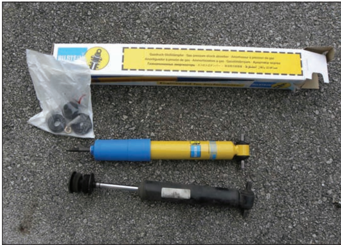
Shock on ground showing bushing and cup washer installation.
