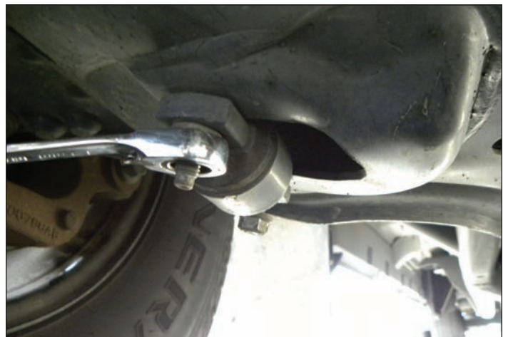
Loosen shock mount studs with a 13mm wrench. With all nuts loose, shock will drop out bottom hole.
