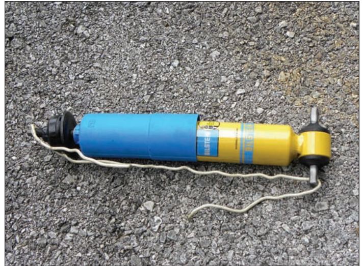
Use a wire to hold shock collapsed to ease installation
