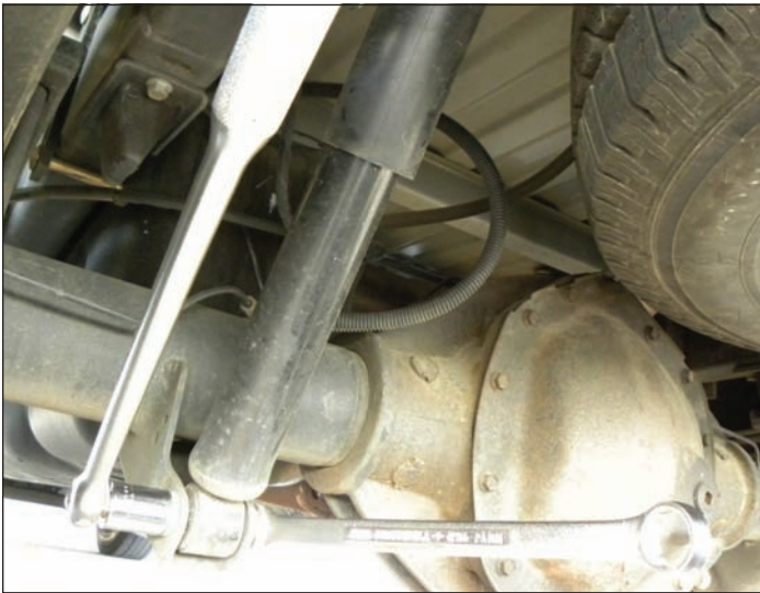
Use open end wrench on bolt head, socket and breaker bar on nut end. Wrench sizes used are different on each shock end.
