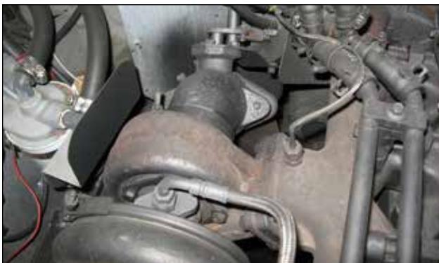
This picture shows a PacBrake installed on a First Generation, manual transmission equipped truck and is very similar to the Jacobs in the positioning of the air cylinder.
