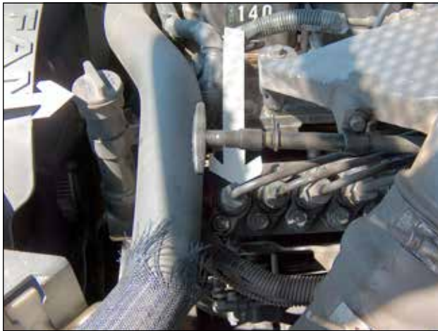
T7. A Bosch P7100 pump on a Cummins B engine, with arrows pointing to the oil filler tube/cap, and to #1 injection line and pump barrel.
