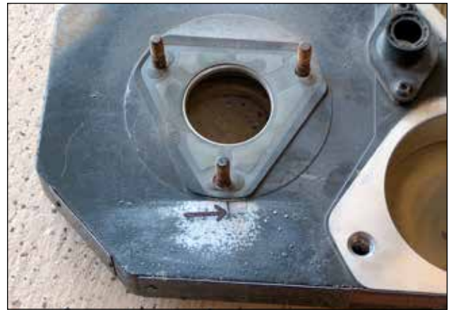
Close up view of the VE pump mounting area of the gear housing with the housing timing mark and the pump-to-housing gasket.
