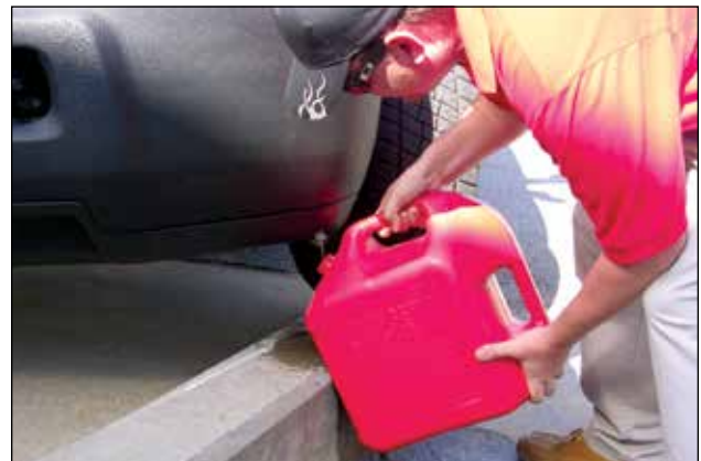
Utilizing the fuel drain line extension tip from Issue 75 it is easy to drain the fuel tank.
