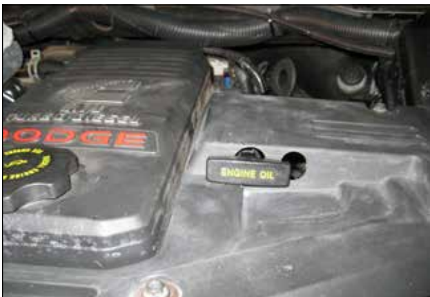
Modified "bat wing" with new dipstick location.
