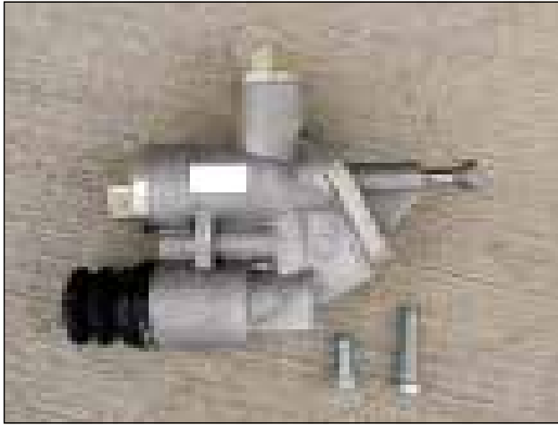
Carter lift pump with regular mounting bolt and longer temporary bolt.
