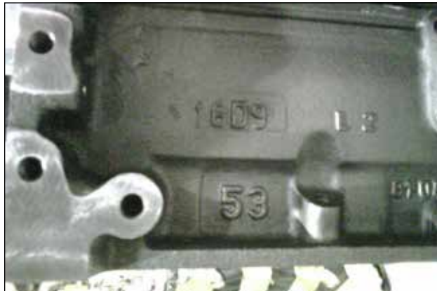
You can't miss it, "block 53," on the driver's side of the engine, toward the front gear case, behind the vacuum pump.
