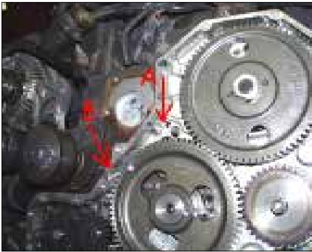
For those not familiar with the dowel pin the arrow shows its location.
