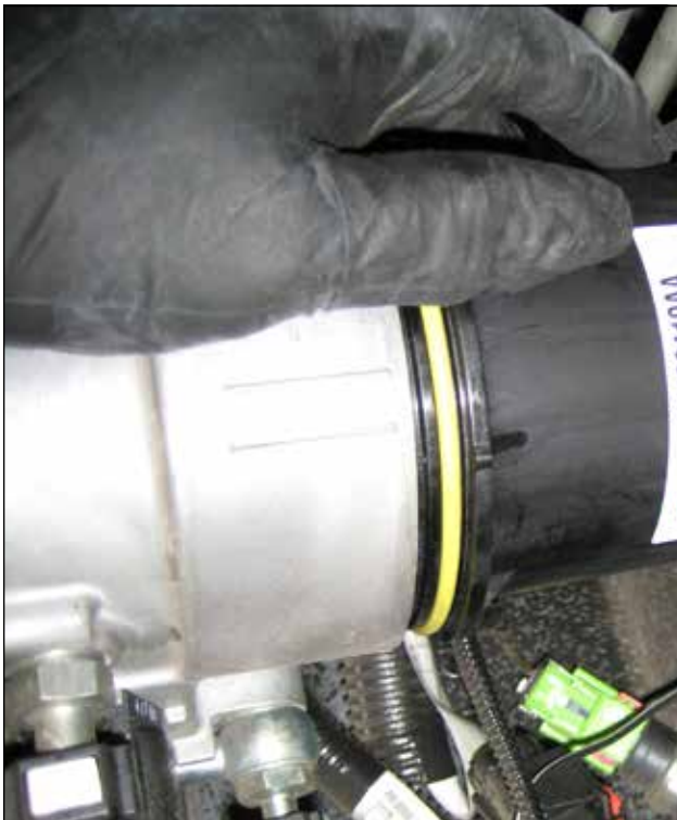
With one hand above and one hand below you can get to the fuel filter from above.
