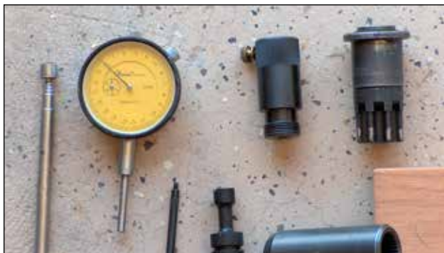
T5. Miller MLR-6860 P7100 pump timing tool kit. At the left is a magnet on a telescoping “stick.” To its right is the dial indicator with the stem extension below and to its right. To the right of that is a timing pin with a steel tip epoxy glued onto it. The special splined socket is at bottom right, with the splined end resting on a block of wood. At top center is the adapter that holds the dial indicator and screws into the top of the pump barrel. At top right is an engine barring tool that plugs into the aluminum block adapter plate and meshes with the flywheel teeth.
