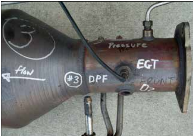
EGT, oxygen and pressure sensors monitor the need for regeneration of the NAC and DPF.
