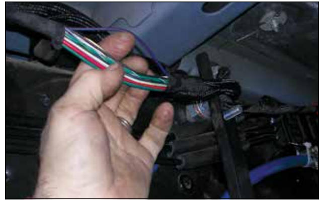
Intercept the wiring harness at the area of the driver's door and you can manually operate the fuel transfer pump.
