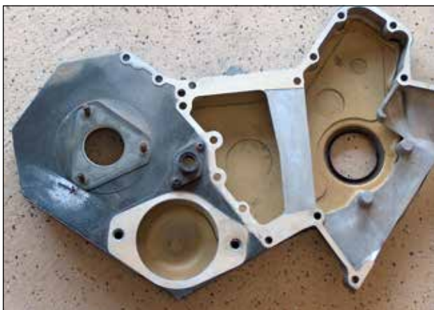
Engine side of a VE-pump style Cummins gear housing.
