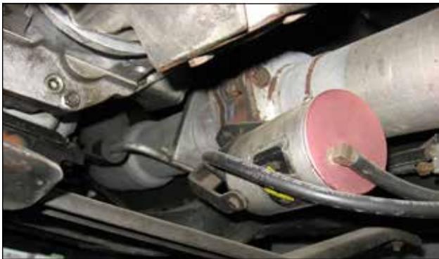
You can see that the inline, under-truck mounted exhaust brakes install in the exhaust pipe instead of directly on the turbo. They are a little more work to install because the existing exhaust pipe must be cut to allow the brake housing to be inserted. They are more exposed to the weather in this location. This one has the flanges nicely welded to the 4" pipe for a leak-free installation.
