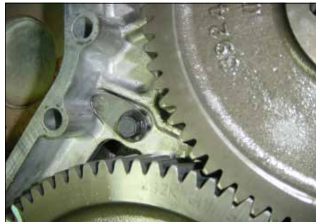
A picture showing an egg-shaped washer that covers the dowel pin.
