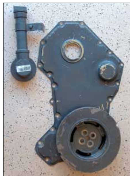
T10. A Cummins gear housing, front side, with the oil filler tube at yop left.
