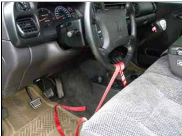
This technique makes the steering stay put while you work which avoids clock spring damage.
