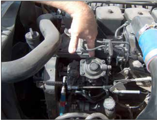
A Bosch VE pump on a Cummins B engine, with a finger showing the clearance between the AFC module and the cylinder head.
