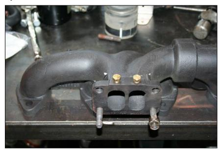
Remove factory studs from the turbo and discard. Install the provided  $M10 \times 1.5 \times 25mm$  (1462431) studs into the turbo.
