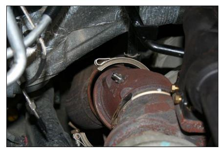
Disconnect the compressor outlet boot.
