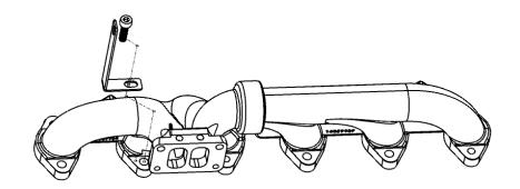
You now have the option to drill a hole through the OEM coolant pipe tab and secure the brackets using the together 1/4 (1100110),1/4" flat washer (1100111), 1/4" lock washer (1100112),and the 1/4" nut (1100113) supplied. Use a 5/16" drill bit to accomplish this.
