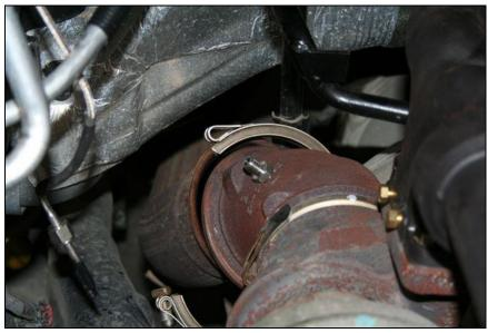
Reconnect the turbo oil drain and oil supply.
