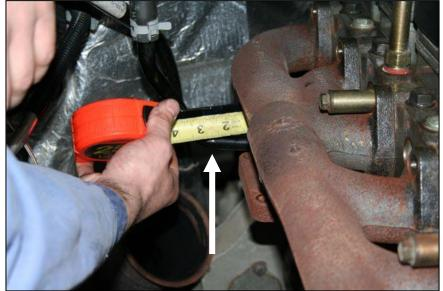
Remove the factory heat shield that covers the front of the manifold.
