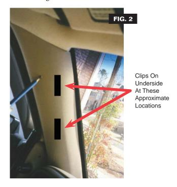
• To route your wires/boost line to the gauges/gauge pod or pillar cover, you will have to remove the plastic A-pillar cover. The cover is held on with plastic clips (Fig. 1).
