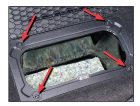
2) Using a Phillips head screwdriver, remove the existing plastic release handle and install the metal "Lock-It-Up" release handle.
