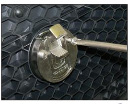
3) Using the metal "L" shape latch (A) as a template, mark its location on the plastic door surround. In order to get more plastic support under the L-latch we recessed the plastic surround by 1/8" inward (B).
