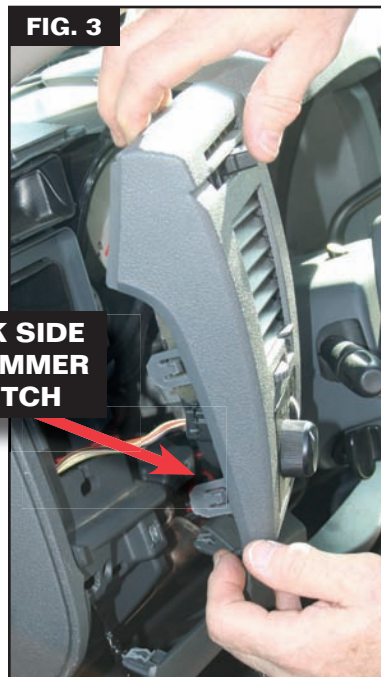
Pull dimmer switch panel back for access to the wiring harness.
