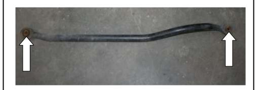
Locate the passenger's side track bar section (#1302030-2F). Thread the 90°grease nipple (#1302056) into thread port on the side of the unit.
