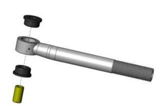
Locate the driver's side track bar section (#1302030-1F). Thread the straight grease nipple (#1302057) into thread port on the side of the unit.
