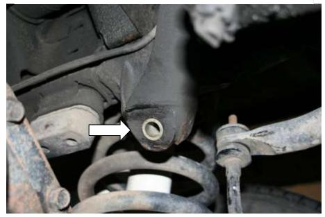
Place the retrofit bracket (#1302001) against the driver's side frame rail, as seen in the picture.
