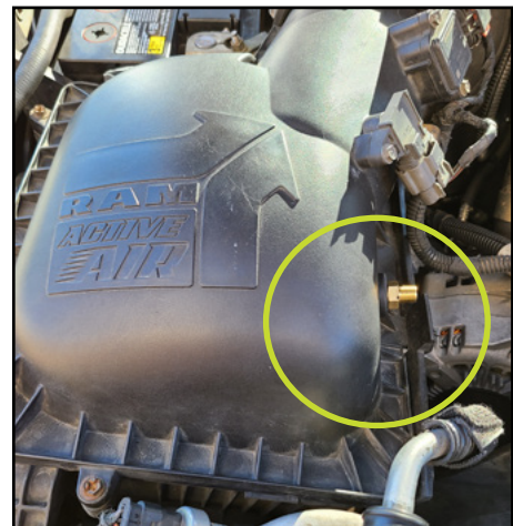
Figure 6: Reinstallation of the air housing and insertion of the barbed fitting
