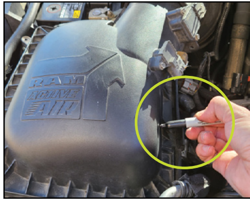
Figure 2: Marking the drill location
