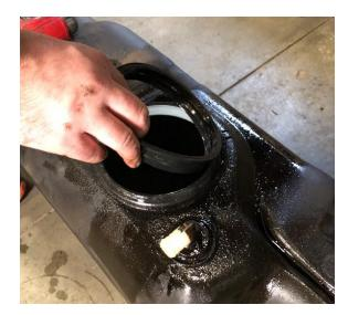
STEP 9: Once the area is clean, install the new seal ring included in the kit into the fuel tank.
