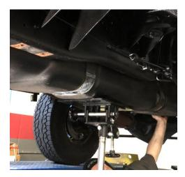
STEP 7: SENDING UNIT REMOVAL With the tank on the ground, make note of the orientation of the OEM sending unit in the tank. The SureFlo sending unit will be oriented in the same manner during installation.
