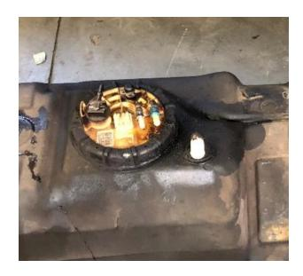
Using a strap wrench, or MATCO tool #FTR730, rotate the sending unit's retaining ring (OE P/N: 52005389) counterclockwise. MATCO tool shown at right for reference. Remove the retaining ring and remove the sending unit assembly from the tank. Have a bucket nearby to catch fuel from the OE unit when removed.
