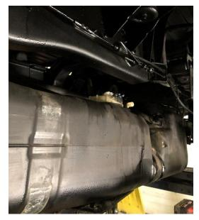
STEP 16: From the driver's side rear wheel-well, connect the electrical wiring harness to the SureFlo. Key on the vehicle and ensure the fuel level is reading appropriately. Start the engine and check for any fuel leaks before operating the vehicle.
