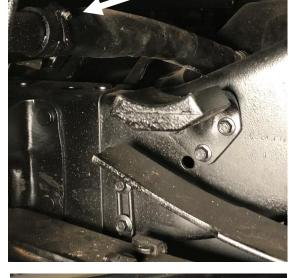
STEP 2: Reaching over the top side of the tank, disconnect the fuel lines and electrical connection for the OEM sending unit.
