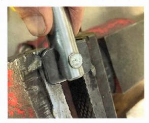
1. Install the supplied 1/8 metal blank in the tube nut as shown and put in a vise as shown. Make sure the blank is supported as close to the tube nut as possible. Insert the knurled pin in the hole and drive it in with a hammer.
