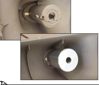
**3) PASSENGER SIDE:** Slide the two larger bushings over the stock plastic mount (this is what breaks)
