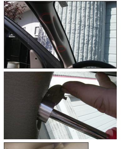
1) Remove Plastic caps with a flat blade screw driver revealing the hidden bolts.
