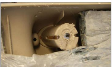
6) DRIVER'S SIDE: You must first trim back the tabs which are protruding from the area in which the larger bushings slides over. This can be done with a pair of side cutters, grinder or file.
