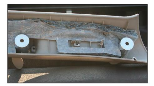
7) Slide the two larger bushings over the stock plastic mount (this is what breaks)
