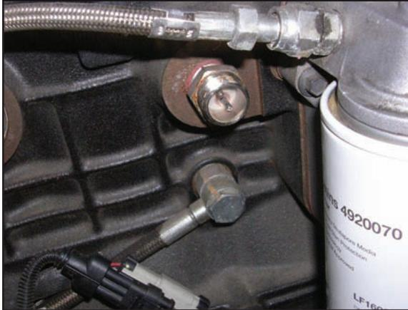
The block heater is located on the passenger side of the engine, about two inches in back of the oil filter. As you can see from the picture on the left, the screw-on plastic cover has been removed and there are two male extensions for the heater cord to plug into.
