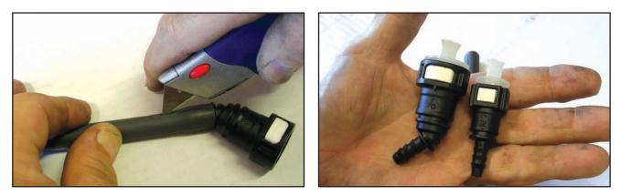
6.) With the clips removed from the plastic line, install the clips into the new hose and the 5/16" pressure tee from the kit into the hose. Tighten the hose clamps and reassemble into place. Take extreme care to keep all of the surfaces free of grit as this hose assembly goes after your fuel filter.
