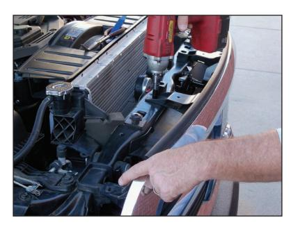
3) Remove the four (4) 10mm coarse threaded bolts that hold the grill in place.
