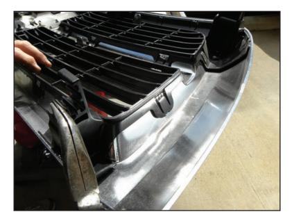
5) Remove the metal clips from the (two on the 2010-2012; all four on the 2013-newer) grill. These clips will not be reused – it is okay to mangle and twist them during the removal process.
