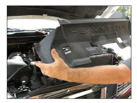
2) Lift the "Heavy Duty" plastic cooling cowl from the radiator core support and set it aside.
