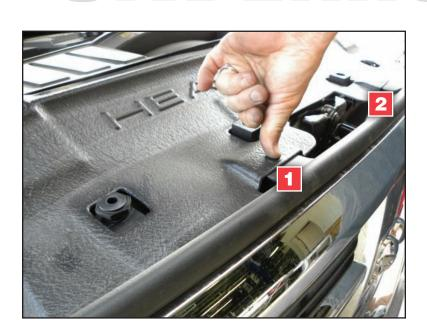
7) Reattach the plastic "Heavy Duty" cooling cowl with the two salvaged plastic push pins.
