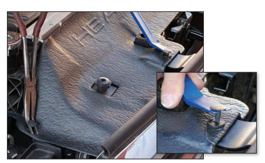
1) Remove the four (4) plastic push pins that hold the "Heavy Duty" plastic cooling cowl in its place. You'll need to salvage two of the four plastic <u>pins</u>.
