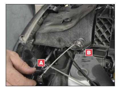
8) With the grill and "Heavy Duty" cowl assembly in position, drop the pins into the outpost holes (A) and (B).
