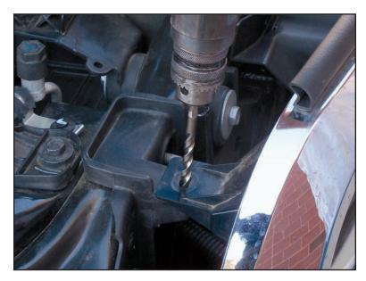
6) Reinstall the grill. With the grill loosely in place, using a 1/4" drill bit, drill out the two "outpost" holes in the grill as well as the plastic that is below the outpost holes. This is done because the size of the factory hole is slightly too small for the pins that will replace the original screws.
