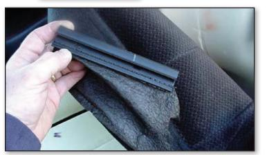
This photo shows the seat back cover's front J-Clip that has been disconnected from the rear J-Clip.
