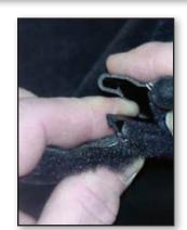
This photo shows the J-Clip that attaches the seat-back cover together as it is unhooked.
