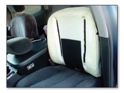
This photograph shows the seat-back cover has been removed. Note the two black strips going vertically up the seat-back cushion. These strips are Velcro, and they hold the seat cover in place.
