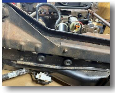
Remove the two T45 bolts holding the gear assembly to the side of the seat track. Try to not rotate the bracket that screws onto the gear shaft. You will want to make sure it is in the same position on the shaft during assembly.
