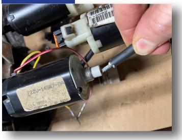
Bend the motor side of the flexible shaft and insert it and the tube into the motor. You may have to rotate and wiggle the shaft to get the square end to engage inside the motor.
