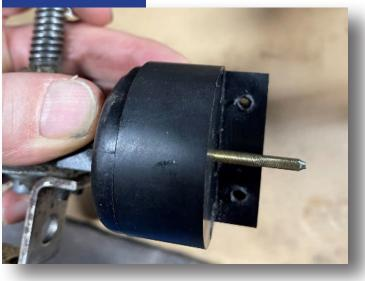
Install the adapter provided in the kit to the gear box as shown. You can insert the flexible shaft later if you want, but when you do, make sure it is fully engaged into the gear assembly. Use the provided #8 screws and #8 lock nuts (9 mm wrench) to fasten it to the gear box.
