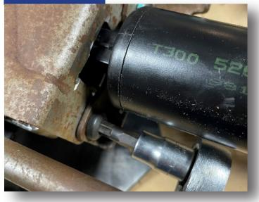
Remove the T45 Torx bolt that holds the gear/motor assembly to the seat frame.
