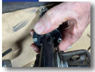
Remove the two screws holding the motor assembly to the gear housing and take the motor assembly off the gear housing. Remove the short flexible drive shaft and put it aside for later. It is used during reassembly so don't discard it.
