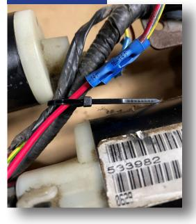
Crimp the butt connectors and secure the for/back harness to the power base harness with the provide zip tie.
