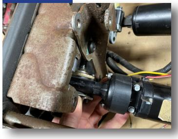
Install the motor/gear assembly onto the seat frame as shown. Make sure the rear vertical lift motor bracket goes under the for/back motor/gear assembly. Install the T45 screw into the bracket and seat frame. Do not tighten it yet.
