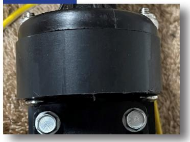
Install the motor onto the adapter. Make sure the square end of the flex shaft is fully seated into the motor. Align the holes on the motor with the predrilled holes on the adapter and secure using the two #8 hex (1/4) head threading screws.
