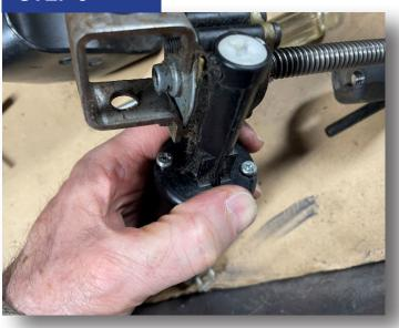
Remove the gear/motor assembly from the seat track.
