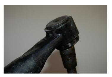
Step 6: If cap does not slide over bar, you must continue to grind until cap slides over, <u>do not force</u> <u>cap over end</u>. Please note
