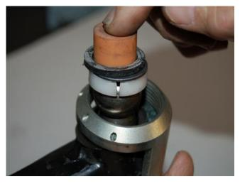
Step 9:Now install the threaded nut and tighten by hand until it wont go further. Then tighten with ½ inch drive ratchet until tight. You will feel it bottom out. This is generally about 35lbs of torque.
