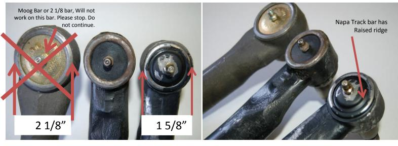
**Moog:** This kit will not work on this bar. This is a 2" diameter bar. Stop and call us for our Exchange program. Dodge NAPA Both these bars are 1 5/8" in diameter across the grease fitting. Go on to next page for installation. Top is Moog, Middle is Dodge, Bottom is Napa. Please note the raised ridge in the encasing seal the grease fitting is screwed into. This is how to identify the NAPA bar. The Dodge bar is flat.
