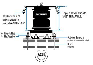
7 Using the 2 "C" clamps, clamp the upper bracket to the frame. If necessary, install the frame to bracket spacers. Ensure the center of the brackets are centered above the axle for correct alignment. Ensure the minimum and maximum distances (from step 6) are achieved and the brackets are parallel to each other. 4 spacer brackets are provided to attain correct mounting height if necessary, install them between the leaf spring and the lower bracket.
