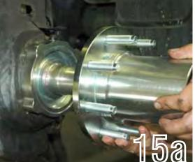
15a -Slide the hub and rotor assembly onto the spindle. Pay close attention that the inner hub bearing seats against the shoulder on the spindle.
