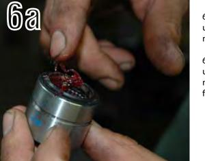
6a -Remove the caps from the ujoint and lightly grease the needle bearings.
