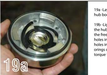
19a -Lay the large o-ring onto the hub body.
