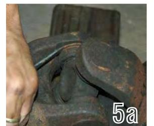
5a -Using a small screw driver and hammer, tap the ujoint retaining clips from the inner axle shaft.
