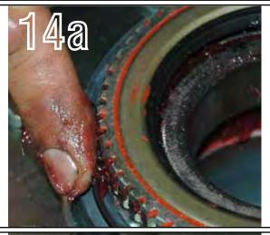
14a -Stretch the v-lip seal over the hub and press the grease seal into the hub after thoroughly packing the bearings with grease. Put a thin film of high quality grease on the lip of the v-lip seal.
