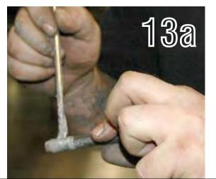
13a -Anti seize the spindle screws before installing.
