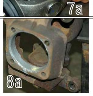
8a -Put a light coat of anti-seize on the knuckle face and bore. This will help with removal later on.
