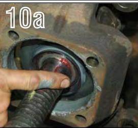
10a -Slide the V lip Seal over the mud slinger as shown. Apply a thin film of grease on the lip.
