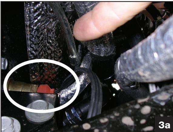
Look up and you'll see the passenger side exhaust manifold heat shield. The block heater element is in the center, directly above the suspension crossmember. For clarity, picture 3a shows the heater cable already plugged in.
