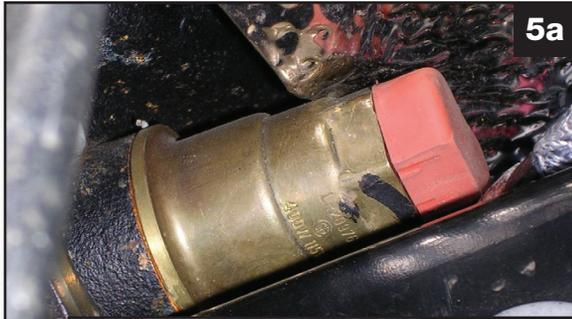
Remove the red dust cap from the block heater shown in picture 5a. Note the orientation of the cap as shown in picture 5b. You will want to hold the heater cord in the same direction as shown in picture 5c.
