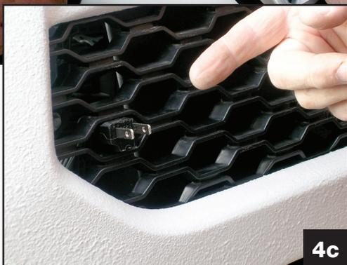
Route the block heater cord over the crossmember and back to the block heater element. Use plastic zip ties along the route to keep the cord away from heat and moving suspension parts.
