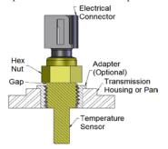
Figure 2: Temperature sensor and harness.
