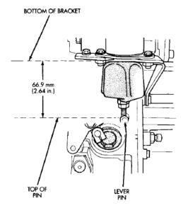
4) If the measurement is not 2.64 inches or 66.9mm (factory specifications), loosen the shaft locknut and rotate the shaft until it is 2.64 inches (Really 2.64, let's try 5/8" or 2.625).
