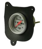
Single A-Pillar mount (PN: GM-DG-01FACE-9902) Mounts in bezel storage compartment.
