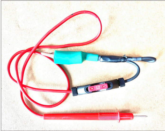
Here it is: Jump-a-fuse to the rescue.
