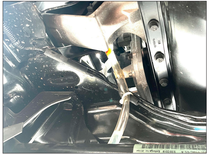
Yes! Scott has extended the factory drain line at the engine-mounted fuel filter.
