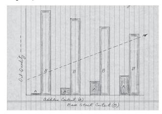
After examining Figure 1 you might conclude that increasing oil quality came about because additive content was increased. This is only partially true. Although additive content and quality are now the most significant contributors to lube oil performance, highly refined base stocks are an integral part of the equation. Higher performance base stocks require a little less additive to correct performance deficiencies, but the base stocks are looking more and more alike.
