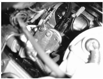
The fuel line to the transfer pump and the fuel line that goes to the fuel tank are pictured here.
