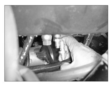
On the inside, the part with the rifled opening attaches the fuel line to the fuel pump. On the outside, the Schrader valve (think A/C valve or, better yet, a tire valve) has a press-for-pressure needle. Here is the catch, you can take the pressure needle out of the Schrader valve.
