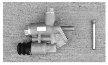
Carter lift pump with plunger removed.
