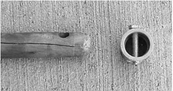
Broom handle, 3/4" coupling with hole drilled and bolt.
