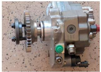
T12. Use of the SP504 gear puller is illustrated here with a Bosch CP3 pump.
