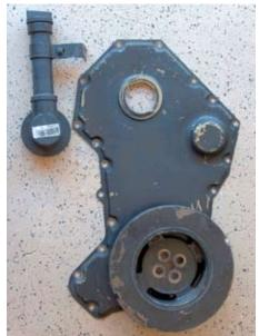
T10. A Cummins gear housing, front side, with the oil filler tube at yop left.
