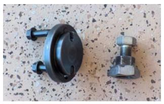
T6. The Snap-on SP504 gear puller with M8x1.25x40 bolts and the home-made pump shaft turning tool at right.
