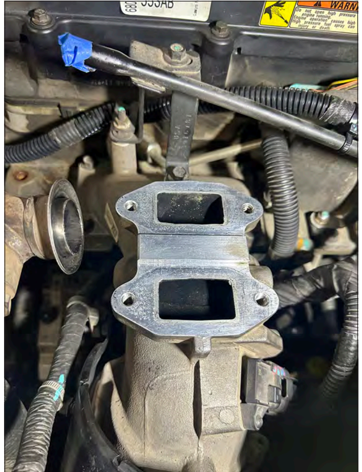
Ready to reinstall the cleaned EGR valve.
