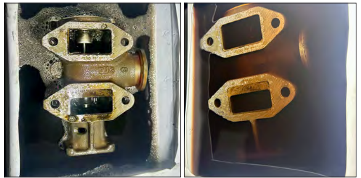
Gallon coolant bottle with one side cutout was used to soak the EGR valve overnight.
