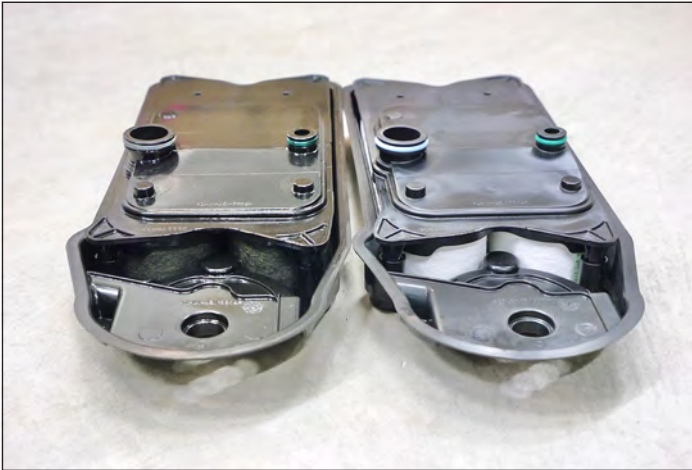
Old CCV filter on the left, new filter on the right.
