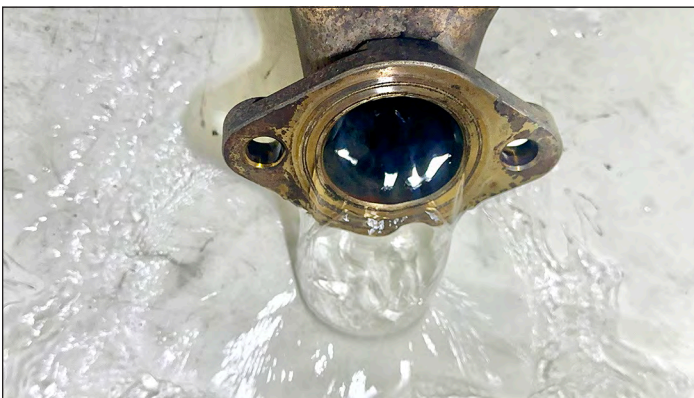
The cooler was rinsed with hot water numerous times, including shaking it with the plugs in-place, until the water came out looking as clean as it went in. Blow compressed air through the cooler to dry it out.
