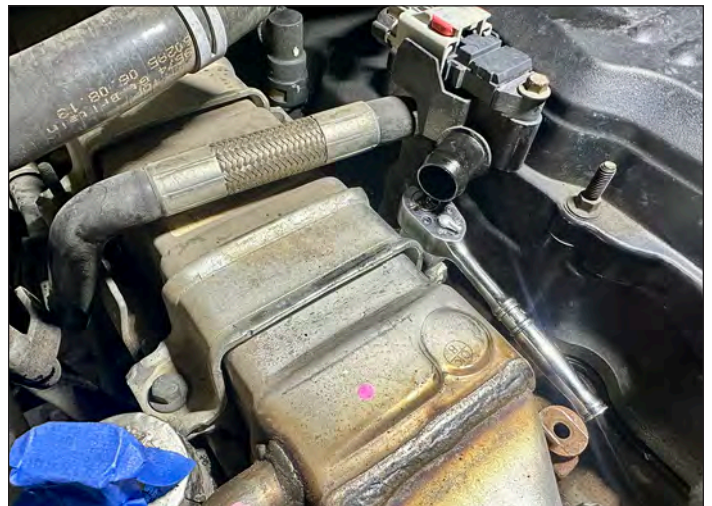
Showing the first of two hoses running over the top of the EGR cooler removed. To disconnect the slightly rearward and partially steel braided hose still attached here, the wiring harness connector and bracket attached the CCV filter/valve cover needed to be disconnected.
