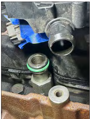
The Geno's Garage parts kit included three new green O-rings. One goes on the end of the elbow-shaped coolant port on the front of the EGR cooler, a second is for the hose with the steel-braided center that crosses over the cooler, and the third is for a hard fitting that sits between the cooler and the valve cover/CCV.
