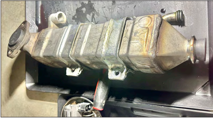
Time for internal cleaning. Note the cooler "plugs" from Geno's Garage.
