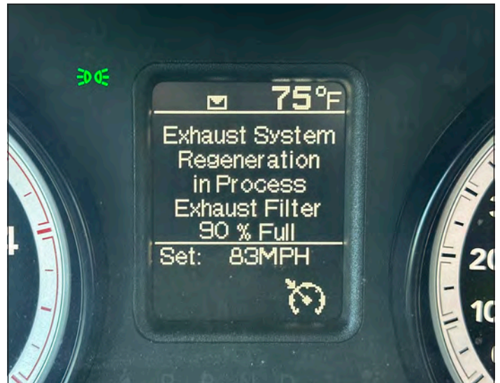
Exhaust filter was full, but after a bit of freeway driving: "Exhaust System Regeneration Completed" was my reward.
