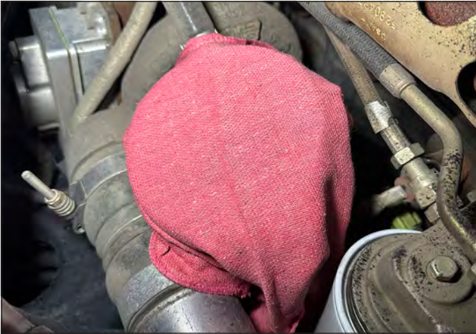
A red shop rag protects the turbocharger intake.
