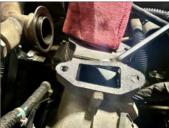
Gaskets below the EGR valve lifted easily, and only a little gentle scraping and chemical cleaning was needed before reassembly.
