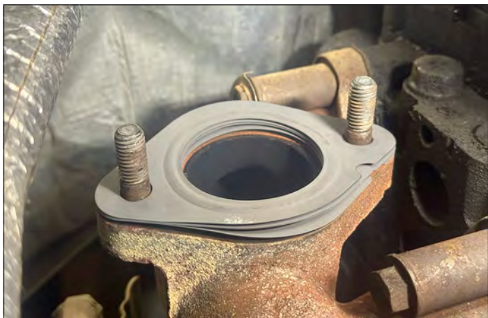
New metal gasket on the two studs for the rear of the EGR cooler before reassembly.
