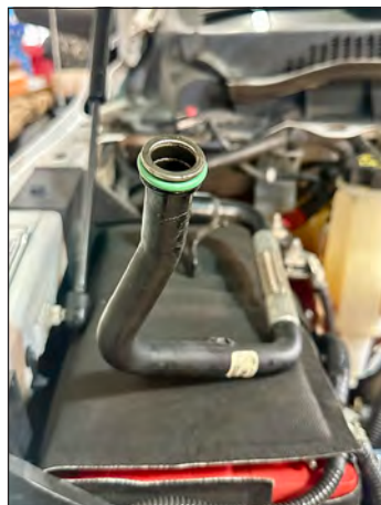
The Geno's Garage parts kit included three new green O-rings. One goes on the end of the elbow-shaped coolant port on the front of the EGR cooler, a second is for the hose with the steel-braided center that crosses over the cooler, and the third is for a hard fitting that sits between the cooler and the valve cover/CCV.
