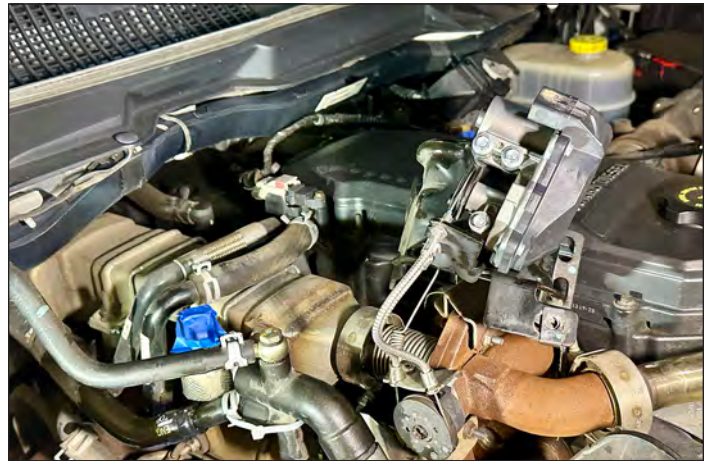
After all four bolts are out, rotate the control valve and bracket toward the valve cover. I held mine out of the way with a bungee cord. There is a spring that might fight you a little.
