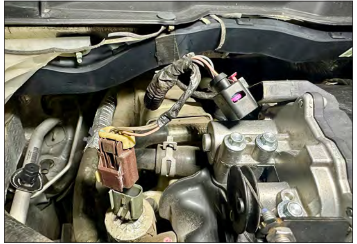
Unclip these two connectors and move the wiring out of the way.
