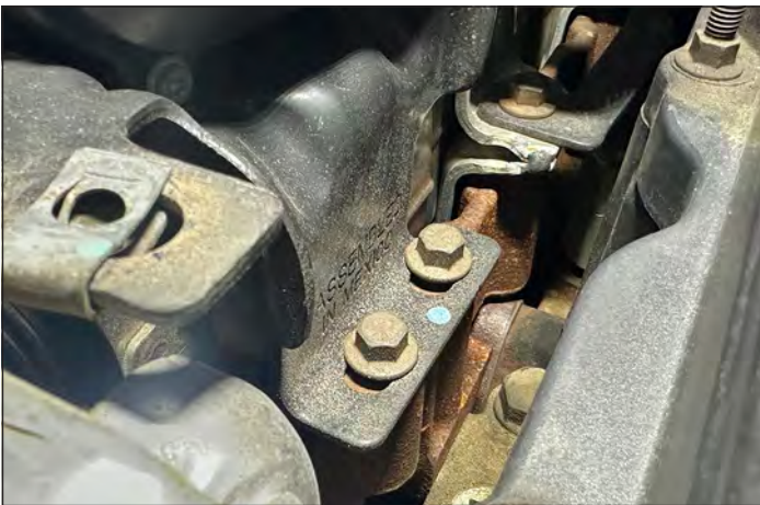
Four bolts secure the EGR control valve assembly bracket to the exhaust manifold. These two, vertical 10 mm bolts are next to the passenger side of the valve cover.
